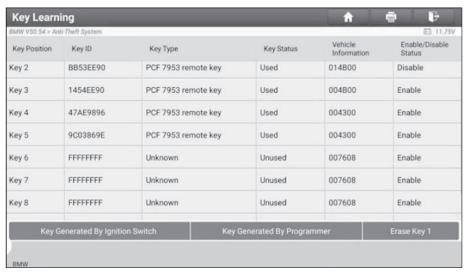
b. Place the new key into the programmer key slot and tap **OK**.
